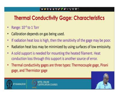
So, let us talk about some basic characteristics or features of thermal conductivity gages the range of such gages is 10 to the power minus 4 to 1 Torr. So, a pressure more than 1 Torr is not measured. Calibration depends on the gas being used, this is because the thermal conductivity is also property of the gas we are talking about. So, the calibration will depend on the gas whose pressure we are measuring.
