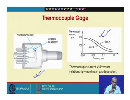
So, this is another diagram for thermocouple gage. You see this is the hot filament and this is the thermocouple, which is welded onto the heated filament. Thermocouple output which is millivolt or you can also take current verses output relationship is non-linear; and it is also gas dependent.
