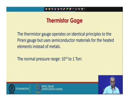
Finally, let us briefly talk about thermistor gage the thermistor gage operates on identical principles to the Pirani gage. So, the working principle is same as Pirani gage. The only difference is that a thermistor gage uses semiconductor materials for the heated elements instead of metals. A Pirani gage uses hot filaments made of tungsten wire or platinum wire or nickel wire; whereas, thermistor gage uses semiconductor material instead of these metals that is the only difference.
