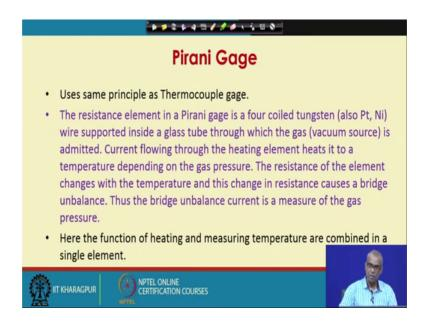
Let us talk about Pirani gage now; another thermal conductivity gage. Pirani gage uses the same principal as thermocouple gage. The resistance element in a Pirani gage is a four-coiled tungsten, you can also take platinum or nickel. So, the resistance element in a Pirani gage is a four coiled tungsten wire or platinum wire or nickel wire supported inside a glass tube through which the gas is admitted. So, the gas admitted is the vacuum source.
