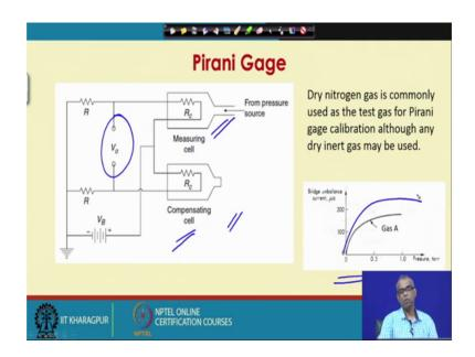
So, this is just another diagram for Pirani gage how will you measure the change in resistance using Wheatstone bridge principle. So, this is the measuring element or the measuring cell to which the vacuum source is connected and this is the compensating cell. So, they are in the adjacent arms. So, this is the output voltage which gives you indication of the pressure of the gas. Dry nitrogen gas is commonly used as the test gas for Pirani gage calibration although any dry inert gas may be used.
