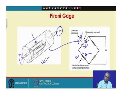
So, this is a schematic of Pirani gage. You can see the four coiled tungsten wire or platinum wire or nickel wire supported within the tube. So, this goes to electrical circuit for heating up the coil, and the gas is admitted or the vacuum source is connected. Now, this is connected to one leg of the Wheatstone bridge.
