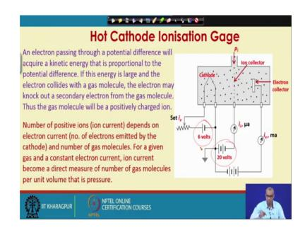
Now, this is the schematic of an ionisation gage. This is the cathode, which is being heated up. So, an electron passing through a potential difference will acquire a kinetic energy that is proportional to the potential difference. If this energy is large and the electron collides with a gas molecule, the electron may knock out a secondary electron from the gas molecule, thus the gas molecule will be a positively charged ion.
