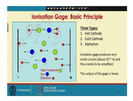
So, let us look at the schematic. Electrons are passing through a potential difference. These are cathodes and anodes. Let us consider this is a close chamber; and to that chamber, the vacuum source is connected. So, we are measuring very very low pressure of say a gas stream. So, there will be gas molecules in this chamber. Now, when the electrons passes through this potential difference, they will acquire kinetic energy which is proportional to the potential difference that is being applied.
