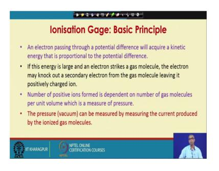
The basic principles of ionisation gage is as follows. An electron passing through a potential difference will acquire a kinetic energy that is proportional to the potential difference through which the electron is passing. If this energy is large, an electron strikes a gas molecule, there is a possibility that the electron may knock out a secondary electron from the gas molecule; and in that case, the gas molecule will be converted to a positively charged ion.
