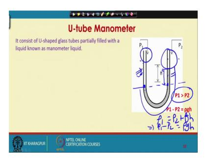
Next, let us talk about U-tube manometer it consists of U shaped glass tubes partially filled with a liquid known as manometer liquid. So, U-tube manometer is U shaped glass tube and this is partially filled with a liquid known as manometer liquid, mercury is a very common manometer liquid.
