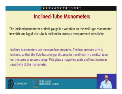
Next, let us briefly talk about inclined tube manometer. The inclined monometer or draft gauge is a variation on the well-type manometer in which one leg of the tube is inclined to increase measurement sensitivity. Inclined manometers can measure low pressures the
