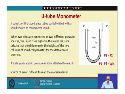
So, when two sides are connected to two different pressure sources the liquid rises higher in the lower pressure side so that the difference in the heights of the two columns of liquid compensates for the difference in pressure. A scale graduated in pressure units is attached to read h. So, a scale graduated in pressure units will be attached from which you can read the h. It may be difficult to read the meniscus level of mercury so that may bring in some error in the measurement.
