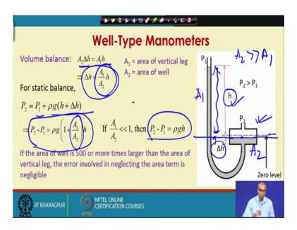
So, let us look at some calculations. So, this is the well time monometer this is the well it has large diameter. Let us say this is the cross sectional area of the well at two this is the cross sectional area of A 1 and A 2 is much much greater than A 1.
