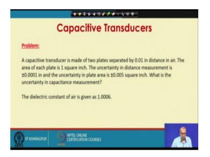
Now, let us take a problem as follows. A capacitive transducer is made of 2 plates separated by 0.01 inch distance in air. The area of each plate is 1 square inch. The uncertainty in distance measurement is plus minus 0.0001 inch and the uncertainty in plate area is 0.005 square inch. What is the uncertainty in capacitance measurement? It is given; the dielectric constant of air is given as 1.0006. So, the dielectric constant is known accurately let us say.
