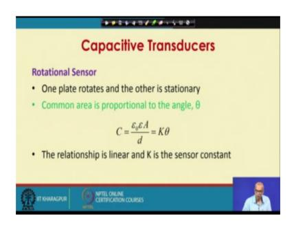
Rotational sensor; one plate rotates and the other is stationary. Common area is proportional to the angle theta. So, capacitance is proportional to angle theta. The relationship is linear and K is the sensor constant and K is the combination of these other parameters.
