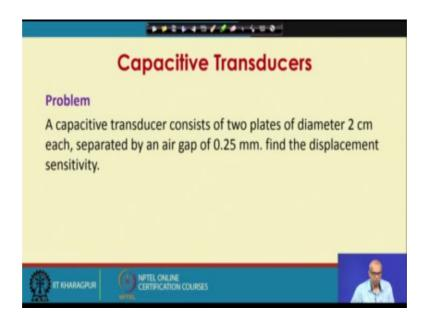
Now, let us consider a very simple problem. I have a capacitive transducer consists of 2 plates of diameter 2 centimetre each, separated by air gap of 0.25 millimetre. Find the
