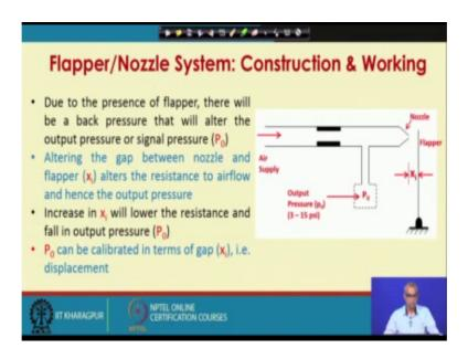
Due to the presence of flapper, there will be a bad pressure that will alter the output pressure or the signal pressure. Altering the gap between nozzle and flapper alters the resistance to airflow, hence the output pressure. Increasing in x I, which is the gap between flapper and nozzle, will lower the resistance and fall in output pressure. So, the output pressure P 0 can be calibrated in terms of gap x I, that is, between flapper and nozzle which is displacement.
