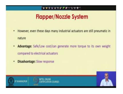
However, even these days many industrial actuators are still pneumatic in nature. So, pneumatic transducer, flapper nozzle system is important component.
