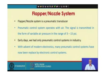
So, let us now talk about flapper nozzle system. Flapper nozzle system is a pneumatic transducer. Pneumatic control system operates with air the signal is transmitted in the form of variable air pressure in the range of 3 to 15 psi pressure. Early days, we had only pneumatic control systems in industry. With advent of modern electronics, many pneumatic control systems have now will replaced by electronic control systems.
