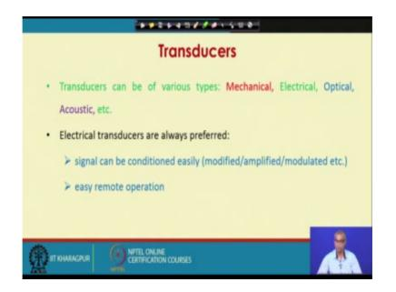
So, transducers can be of various types; mechanical type transducers, electrical type transducers, optical type transducer, acoustic type transducer so on and so forth. Electrical transducers are always preferred, because the signal can be conditioned easily; that means, signal can be modified, amplified, modulated etcetera. The remote operation is easy; that means, the signal can be transferred from one place to another very easily.
