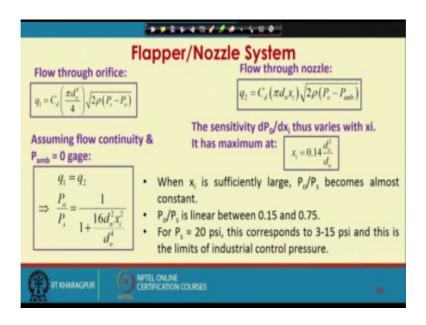
So, flow through orifice can be expressed by this equation. So, we consider flow through orifice as  $q \ 1$  and  $q \ 1$  can be expressed by this equation. P s is the supply air pressure and P o is the output pressure. So, P s and P o represent the pressure drop across the fixed flow restriction which is orifice.
