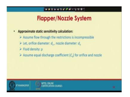
Now, let us see how we compute approximate statistic sensitivity for a flapper nozzle system. Assume flow through the restrictions is incompressible. So, we consider incompressible fluid flow. Let the orifice diameter be represented by d o and the nozzle diameter be represented as d n. Fluid density equal to rho. Let us assume equal discharge coefficient C d for orifice and nozzle.
