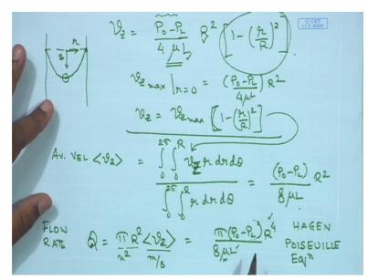
So you measured the Q, the amount of liquid that you are collecting per unit time and if it is falling freely vertically then p0 minus pL can be substituted just by the gravity force. You need to know the diameter or the radius of the capillary, the length is known, so thisyou are going to find out experimentally. All these are known to you. The only one known here is the property mu.
