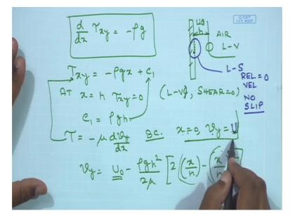
So the belt pulls the liquid, the gravity tries to drain the liquid. A steady state is reached with the condition that the velocity on the belt on the liquid side would be equal to the upward
