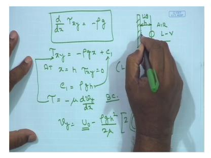
So at the liquid-solid interface, the relative velocity is zero. Which is initially we call it as no slip velocity. Since it is no slip,the velocity must be equal to the velocity X is equal to zero, must be equal to the upward velocity of the belt.
