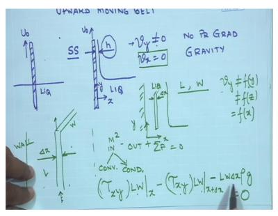
So the next step is simply divide both the sides by del x, taking the limit and obviously cancel LW from all sides. Divide both sides by del x and taking the limit points del x tends to zero.
