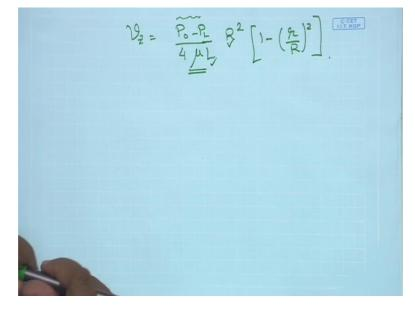
And it is obviously then the velocity distribution because of the nature, because of its R dependence, the velocity (dep) is going to be parabolic in nature. So this is your R and Z. So
