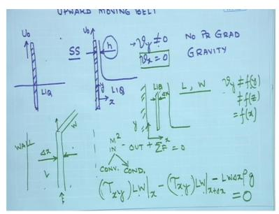
So you see how easy it is now to write the difference equation. It is progressively becoming it easier for you to clearly visualize the flow condition. Write the governing equations. Get rid of all the terms which are not relevant. For example in this case the transport of momentum by convection by flow. Since the velocities are same at the bottom and at the top. So no net contribution of momentum.
