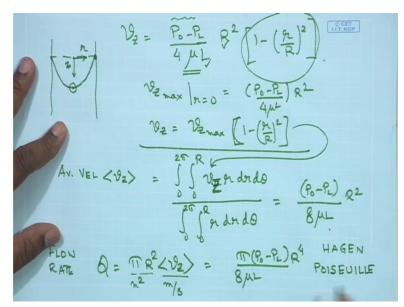
So this HagenPoiseuille equation gives you the volumetric flow rate for a fluid which is flowing through a vertical tube because of the presence of a (velo)pressure gradient and body force. So this is the imposed condition, this is a geometry, these two other geometrics and this
