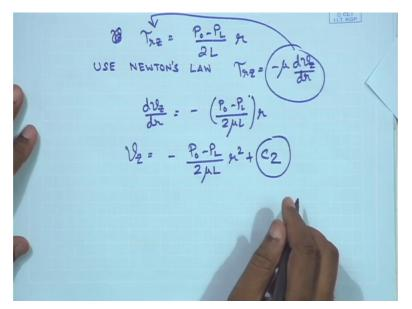
So how do you evaluate C2? You need a boundary condition and the boundary condition that is available to you is, no slip at small r equals to capital R. Because in this shell, when smaller becomes capital R then you essentially have a liquid-solid interface and at a liquid-solid interface, the relative velocity is zero. So you would have vZ is equal to 0 at small r equals capital R.
