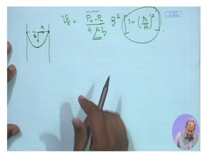
So this is the point of maximum velocity and from the expression you can simply see vZ max is essentially at R equals to 0, at this point, which would simply be equal to p0 minus pL by 4 mu L timesR square. So we can write vZ as vZ max times 1 minus r by R whole square. The expression for vZ can also be written in this way.
