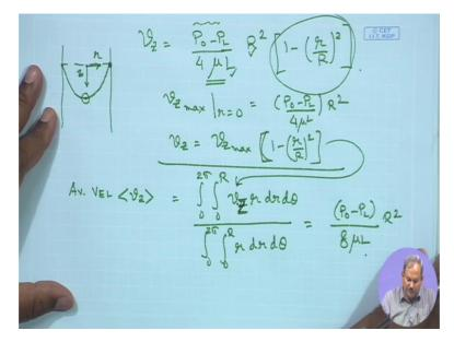
And once you have the average velocity, the flow rate Q would be equal to pie R square times the velocity. So this is meter square, this is as units of meter square, this is meter per second. So this together it becomes meter cube per second which is volumetric flow rate which would be equal to pie p0 minus pL by 8 mu L times R to the power 4. This is a famous equation which is known as the Hagen Poiseuille equation.
