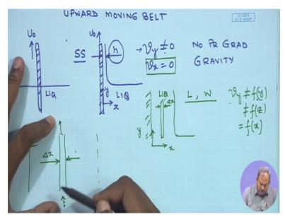
So I do not need to write, when I write the momentum in minus out plus sum of all forces is equal to zero and I identify there's going to be a convective part and there's going to be a conductive part. The convection part, I do not need to write since the velocities at these two points are equal. But I need to take into the account the tau. Now what is going to be the subscript of tau? The subscript of tau, the first subscript would be the direction in which the motion is taking place.
