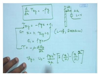
Now you can see that it is slightly more (comp) complicated than the simple parabolic distribution profile. You have a linear term and you have a quadratic term and you have the velocity with whichthe belt has been pulled up. The second boundary condition would be at X is equal to zero. Your vY must be equal to U. This is a very important boundary condition.
