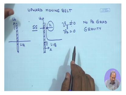
So if that's the case, then we would like to find out what's going to be the velocity distribution, vY in this case, in the thin portion of this liquid.
