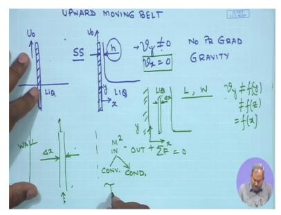
So if you seethis basic problem, the motion is upwards in the plus Y direction. So the first subscript of the shear stress in this case is simply going to be tau Y and as a result of motion in the upward direction and variation in velocity, the momentum gets transported in the X direction. So the subscript of tauwould be tau XY in this case. Y momentum gets transported in the X direction. So tau XYthis is going to be the shear stress.
