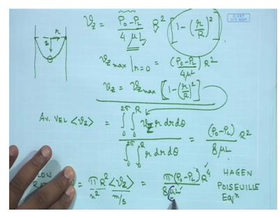
So using a capillary viscometer where a very thin capillary is used to obtain some flow out of the capillary, the only unknown being mu. Mu can be calculated. So that is the principle of capillary viscometer. Whenever we (ha) get such an expression, we need to be careful about what are the assumptions we have made because we need to know the assumption in order to get an idea of the applicability, the reason of applicability of in a relation or a correlation that we have developed.
