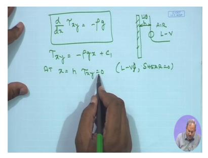
So you C1 would be simply equal to rho GH. And also tau, if I assume it's a Newtonian fluid, it is simply going to be mu timesd vY by dX and this D vY by dX in using plugging in this in here and using the value of C1as rho GH,you can integrate this. I am leaving it for you to do.
