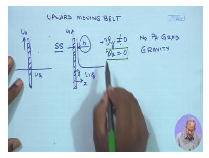
So in order to obtain the shell, if this is my wall and this is the liquid film and this is X and this is Y, then my shell must be something which is of thickness delta x. It could be any length L any width Y, does not matter. Because vY is not a function of Y, it's not a function of Z, it's only a function of X. So that's why Iam taking my shell as this.
