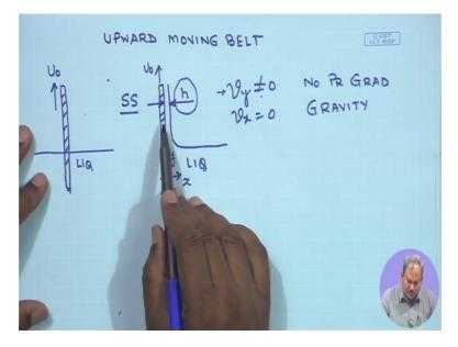
So we have to think of a shell and in order to think of a shell we need to first identify what is the direction in which the velocity is varying. Because whatever be that direction, that's going to be the smaller dimension of the control volume. You can clearly see that the velocity is varying with X. this is moving upwards, this is a free surface, the velocity does not vary with Y and there is no vX in here.
