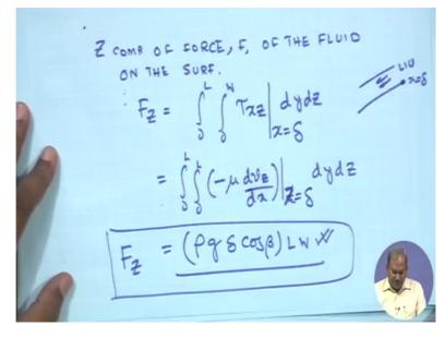
So Z component of force, let us call it as F of the fluid on the surface, it is in the Z direction from 0 to L, from 0 to W tao XZ, remember that we have to evaluate this shear stress at at X equal to delta because that is where it is acting. This is the liquid and this is that X equal to delta dY dZ. So this is the same as for tao - mu Times d VZ dX at Z equal to, sorry at X equals delta dY dZ, it would be equal to rho G delta cos beta L times W. This is the force in the X direction.
