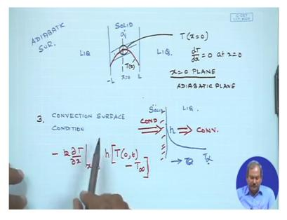
And the 3<sup>rd</sup> condition could be that I have a convection surface condition where you have surface which is solid, on this side you have a liquid let us say and the profile of temperature is this where you have T infinity, the temperature over here is T infinity and the heat transfer coefficient involved is H. So heat will come from here to here by means of conduction and from here to out by means of convection.
