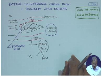
But let us look at this figure first, what we have drawn here is, this is an air foil which is moving, which is moving in air, and you have the air, this is moving so the upstream velocity, you can think of this as a relative velocity, U infinity with which the air approach the air foil. At this point, is the stagnation point, so these are streamlines of the liquid, which forms around the air foil. And the point at which the, it hits the air foil, is called the stagnation point.
