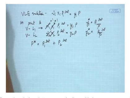
We assume for a time being that we are dealing with low pressure systems, for low pressure systems it's the standard VLE relation which we have written n number of times in our entire course is given by gamma i Xi the standard relation this is equals to yiP. Now if we apply this relation to the point B say, at point B, what is there? We find at point B vapour is in equilibrium with liquid L1 and vapour is in equilibrium with liquid L2.
