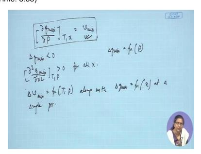
We need to have this particular information along with Delta g mixture as a function of x at a single pressure only if we have this data we can find out that under what conditions the 2 components will be mixing under what conditions the 2 components will not be mixing? They will be forming immiscible systems and if by increase of pressure we would land up into a miscible system or an immiscible system it all depends upon the sign and magnitude of the volume change of mixing of the 2 liquids.
