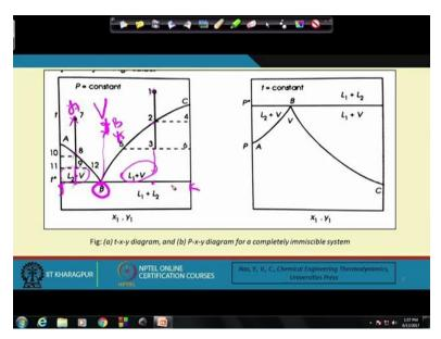
And we observe one more interesting thing we find that at any particular specified pressure say for example this phase diagram is drawn at a constant pressure for such a case if 2 immiscible liquid phase is are in equilibrium with the vapour phase we find that the 3 phase equilibrium temperature will always be less than the saturation temperature of either liquids at that pressure, is it clear?
