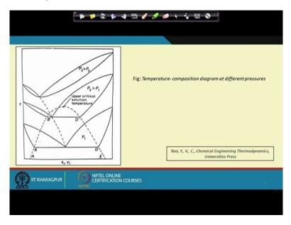
Now suppose we have drawn it at one particular pressure, suppose we would like to repeat the experiments and see what happens if we are if we are drawing this Txy diagram at different pressures, what do we find if we go for higher and higher pressure? There are 2 things that we observe first thing is the T star which we have seen the T star it keeps on increasing as we increase the pressure or the 3 phase equilibrium temperature as it is called that increases as increase the pressure.
