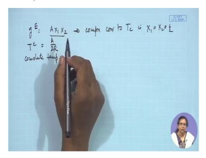
And we also find that if gE is given by this equation then usually the composition corresponding to Tc is given by X1 equals to X2 equals to half but usually we find that gE is not given by such a symmetric distribution or gE is usually not so very symmetric with X1 and X2 and therefore the coordinates of the consulate point is often not at the composite midpoint. Well there is one more interesting thing that I would like to point out and we will be discussing it in the next class.
