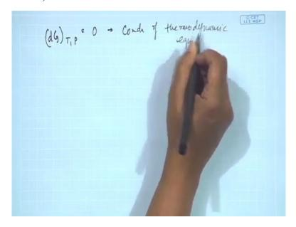
Or in other words mathematically if we put it we have seen that the condition of thermodynamic equilibrium under conditions of constant temperature and pressure is given by this particular equation, okay. And therefore it is quite evident that when there are 2
