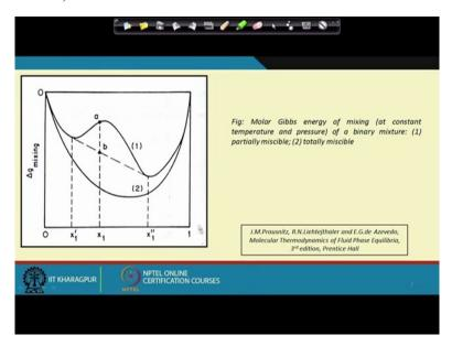
For example this particular situation is given by curve 2 in this figure. In this particular curve we find that a single liquid phase will be obtained over the entire range of composition starting from X1 equals to 0 to X1 equals to 1.
