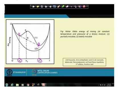
Just the curve which I have shown in this particular figure and here we find that as I have already discussed for a completely miscible system the Gibbs free energy of mixing always reduces it is always less as compared to the Gibbs free energy of the individual components. Now under certain conditions if it happens that on mixing instead of following curve 2 the solution or rather the mixture it follows curve 1.
