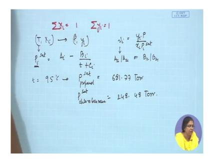
T equals to 95 degrees centigrade we already know, right? And then once we know this it's a binary mixture, we are in a position to find out the saturated pressure of propanol the saturated pressure of chlorobenzene if you calculate this you will be finding that the saturated pressures are 681.77 Torr you can check it up just see that units etc are consistent otherwise there is no place where you can make a mistake, right?
