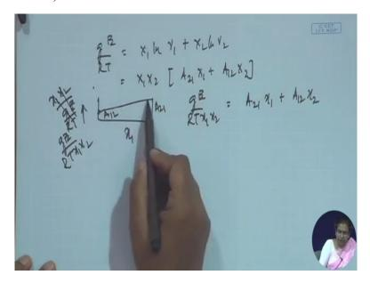
What is the way of combining ln gamma1 ln gamma2? If you recall the original expression of g by RT, what was it? g by RT was equal to if you remember it is nothing but X1 ln gamma1 plus X2 ln gamma2, isn't it? So what can we do for this particular case? We can write it down as if you substitute the expressions of ln gamma1, ln gamma2 then in that case we find that this will be equal to X1X2 A21 X1 plus A12 X2, right?
