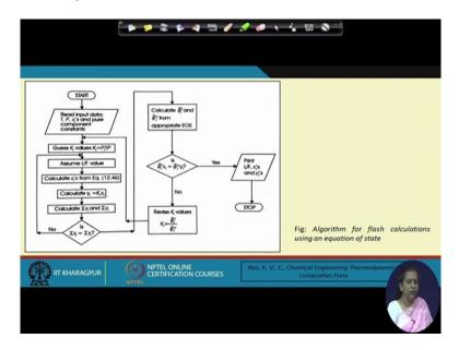
And also for the Flash calculations, right? So therefore you can use this particular algorithms and you can you can find out the VLE data at high pressure and the VLE data for multi-component system remembering very well that the VLE data at low pressure that has been discussed for binary systems is applicable in this particular case.
