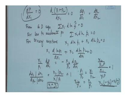
That for this particular situation can we not write down dP by dX1 equals to 0. What is this P? It is just the summation of the partial pressures, so therefore we can write it down in this particular way. From where we can write down dP1 d X1 is nothing but equal to dP2 d X2,
