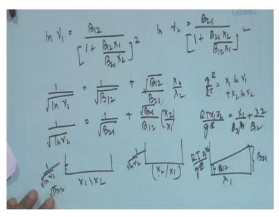
So in this particular case just look at the equation, can we write it down in this form? Say suppose if we can write it down as ln gamma1 which is equal to I will just write down the equation once more it was B12 by 1 plus B12 X1 by B21 X2 whole square and this was ln gamma 2 it was B21 by 1 plus B21 X2 by B12 X1 whole square. Just these 3 equations it will be good if you can remember them, agreed? So therefore can we just write it down in this particular form?
