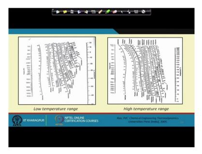
Yeah, so several K plots are available for different pressure and temperature conditions at low-temperature range and high-temperature range from which K can be found out and the VLE at high pressure can be worked out accordingly.
