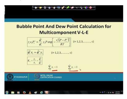
And well the bubble point and dew point calculations we have been discussing for binary mixtures, if you're going for multi-component VLE data the same procedure is going to apply just we need to remember that instead of working with 2 components we will be working with more
