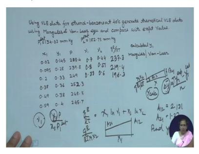
So therefore in a very similar manner if we take up this particular data. Here in this particular case also you can very well from here again find out gamma 1 gamma 2 gE by RT is the same then instead of this particular thing in, here you need to plot X1 X2 by gE by RT as a function of X1 and then from the intercepts you are in a position to find out B12 and B21, once you
