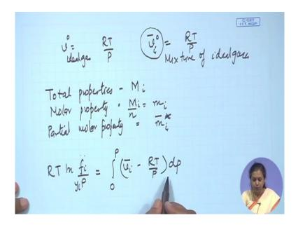
In the same way, so I will just repeat it once more in the same way v for an v0 ideal gas naturally 0 means ideal gas that is equal to RT by P. Interestingly suppose this same gas it is in a mixture with other gases where I have to define the partial molar volume just note the partial molar volume since it is molar it is small case it refers to component i subscript i, it refers to the ideal gas state superscript 0 this is a partial molar volume there is a bar.
