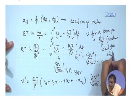
So in other words we would like to express aij in terms of aii and ajj and this was possible by means of combining rules so we have devised a number of combining and mixing rules and
