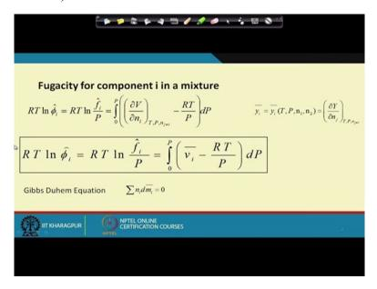
So therefore from this particular equation from this particular equation what are the things that we see? We see from this equation that more or less the fugacity of component i in a mixture it is something different from the fugacities of or rather it is different from the other partial molar volumes number 1.
