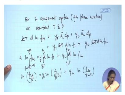
Say for the time being just for simplicity for 2 component system which is gas phase mixture at constant temperature and pressure. If I elaborate that what do I get? RT d ln fM this is equals to y1v1 bar dp plus y2v2 bar dp, agreed?
