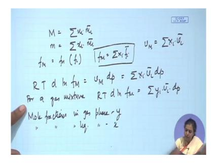
Now what is that equation? What is the basic defining equation RT d ln fM which is the fugacity of the total mixture that is equal to vM dp, right? This one we know. What is vM equals to? Just if we can write it in this particular terms v mixture is nothing but Sigma xi vi bar, fine. So instead of vM can I not write it down at as xivi bar dp, fine.
