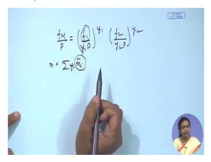
Or in other words for removing the ln terms what do we get? We get fM by P this is equal to f1 by y1 P whole to the power y1 f2 by y2 P whole to the power y2, is it clear to you?
