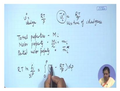
That in order to calculate fugacity we need to know the partial molar volume of component i in the mixture not only at the pressure of interest but since it is inside the integral we need to know this particular value or how this varies with pressure right from P equals to 0 to the pressure of interest, right?
