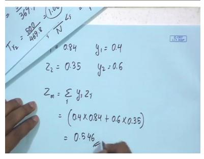
So here we know we have (calculated) we have proved it earlier for Amagat's law Zm is equal to summation of yi and zi. Here y1 here we know mole percent of propane is 40 and mole percent of n-pentane is 60, so y1 is 0.4 and y2 is 0.6. So we simply do the summation here 0.4 into 0.84 plus 0.6 into 0.35 and we get the value of Zm as 0.546.
