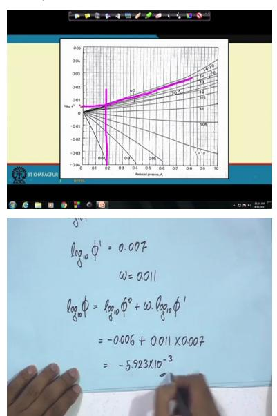
And in the same way we need to find out the value of log phi 1, we go to the next chart we start from 0.2 that is this point, so 1.6 curve is here it meet somewhere here and we get the value of log phi 1 as 0.007. So we know these two values, we know the value of acentric factor. So log phi and we get the final value of log phi as minus 5.923 into 10 raised to minus 3.
