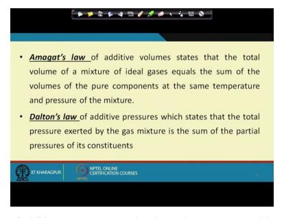
So Dalton's law of additive pressures states that the total pressure exerted by the gas mixture is the sum of the partial pressures of its constituents.
