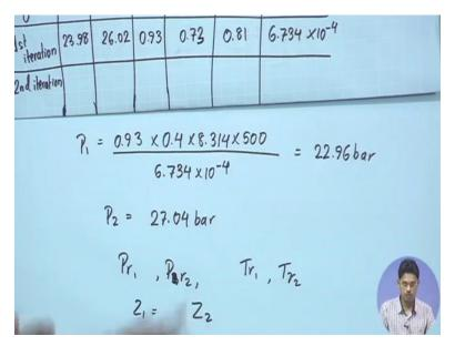
Now as we have got the value of Vm after our first iteration, so we need to do our second iteration. So we need to calculate P1 and P2 again from the new values of Z1 and Z2. So I am going to that here. The new value of Z1 is 0.93 and the new value of Vm is 6.734 into 10 raised to minus 4 and we get the new value of P1 as 22.96 bar, similarly we get the new value of P2 as 27.04 bar.
