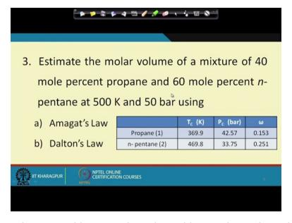
So we move onto the next problem, I read out the problem. Estimate the molar volume of a mixture of 40 mole percent propane and 60 mole percent n-pentane at 500 Kelvin and 50 bar using one Amagat's Law, two Dalton's Law. So the values of critical temperature, critical
