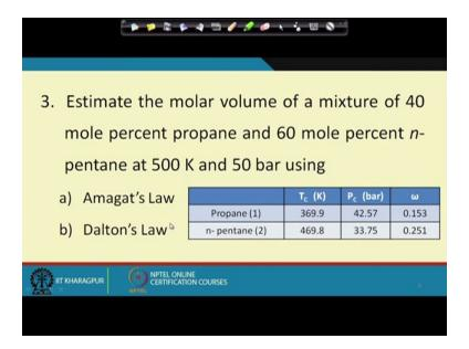
So we get the value of Vm value of Vm that is measured is 4.539 into 10 raised to minus 4 meter cube per mole, okay. Now we need to go to the second part of the problem that is the estimation of the molar volume of the mixture using Dalton's Law.
