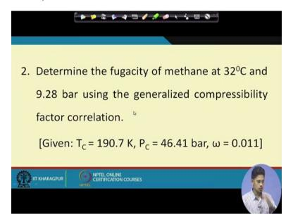
So I am going to do a similar problem that is our second problem, I am going to read out the problem determine the fugacity of methane at 32 degree celsius and 9.28 bar using the generalized compressibility factor correlation. The Tc, Pc and acentric factor values are given. So we proceed in the same way we did in the last problem.
