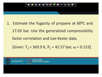
So let me go to the problem first of all. So the first problem I am going to read it out, estimate the fugacity of propane at 60 degree celsius and 17.03 bar. Use the generalized compressibility factor correlation and Lee-Kesler data. So the critical temperature and critical pressure are given Tc is equal to 369.9 kelvin and Pc is equal to 42.57 bar, the acentric factor is given and it is 0.153.
