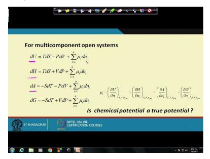
So therefore this can also be written down as del U del S at constant v, n ds plus del U del V at constant s, n dv plus Sigma i equals to 1 to n mui dni, right? Where each mui it corresponds to del U del ni of the ith component where the number of total number of moles of all other components except the ith component is kept constant, I have written down the equations for the multi-component open systems in each case.
