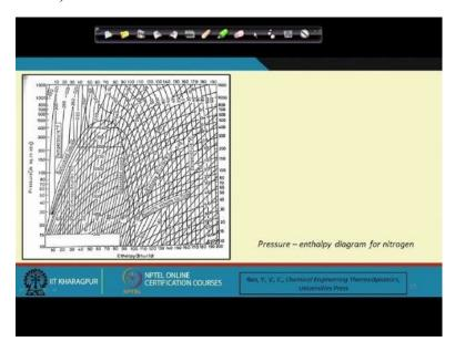
A few of these are the pressure enthalpy diagram which is shown here, these Particular diagram is shown for nitrogen and here if you observe we will find that the entropy curves are given the pressure and enthalpy I have given and we also have the specific volume data and the temperature data. So therefore it contains large number of data and we have been in a position to find out the enthalpy and entropy we can have such particular charts for other gases as well.
