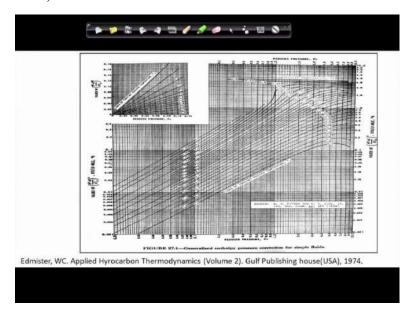
We should be able to generate Delta s star by R curve as a function of unique functions of Tr and Pr and this has been done by a large number of researchers so long and the curves they are of this particular form. These curves they have been generated by Edmister and they are used very frequently in the hydrocarbon industries in order to estimate the reduce enthalpy departure function as a function of reduced pressure and a function of reduced parameter, okay.
