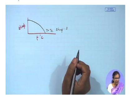
Or in other words, suppose I plot delta h vaporization as a function of temperature then what is the curve which I expect? It should have a high latent heat vaporization to start with it keeps on decreasing and then at T equals to Tc we find delta h vaporization equals to 0, fine.
