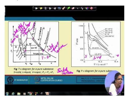
On the contrary if the triple point pressure is much less than the atmospheric pressure then at atmospheric pressure what are you doing basically? You are operating in this particular region where you find that the solid will be converted to the liquid and the liquid then will be converted to the vapor and this gives you the answer to questions as to why some substances sublime.
