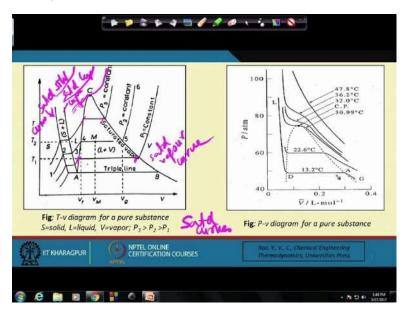
This is what I have shown in this particular figure if you see I have tried to show this, this is for carbon dioxide. Now there is one thing I have already told you about the point of termination of the liquid vapor curve, right? Liquid vapor dome, sorry, this is nothing but the critical point, what about the initial portion? Where does the liquid vapor dome or in other words where from where do this saturation curves they originate?
