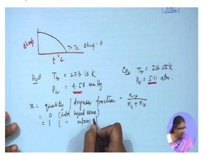
We know what is x equals to? x is nothing but the quality or the dryness fraction, right? What is this quality or the dryness fraction? Suppose they're working with nv moles of vapor nl moles of liquid and then nv moles of vapor, okay. So therefore we know that this is equal to 0 as I have already mentioned because nv equals to 0 on the saturated liquid curve no matter what pressure or temperature you have operating equal to one over the saturated vapor curve.
