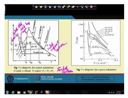
We can construct such isobars at different pressures, right? And this is what precisely I have done here. We have constructed isobars at different pressures at increasing pressures and we find that we get such identical curves as I have already shown.
