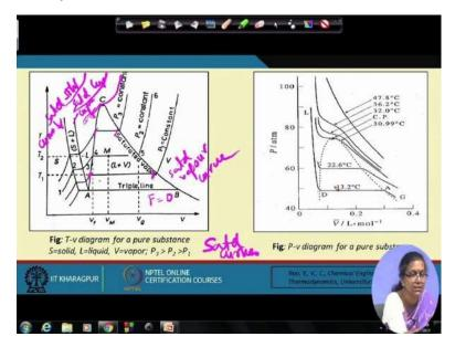
If you observe this data what do you find? You find that the triple point curve for carbon dioxide this particular curve here as well as here this occurs at a pressure much higher than the atmospheric pressure.
