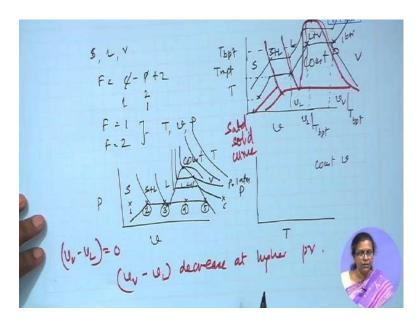
In the same way we can plot our Pv diagram also, we are going to start in the similar fashion that we have done here we take our substance we start heating it and then as we heat it at constant pressure initially the substance was here we heated the pressure remains constant it is here and then it changes to the vapor phase, sorry liquid phase then the liquid gets heated and then it goes to the vapor phase and then the vapor is heated to a very high temperature.
