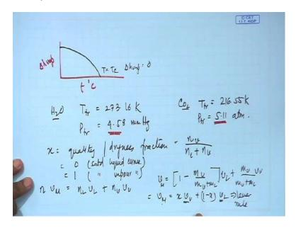
Suppose we are at this particular position by measuring the horizontal portions, we can find out x and 1 minus x and we already know these 2 so we can find out yM from here
