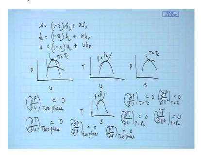
And here I would like to mention that the similar relationship this additive property in fact this holds for all extensive properties of pure substances we can have s equals to 1 minus x sL plus xsv similar way we can have the same thing for enthalpy the same thing for internal energy and so on and so forth we can keep on having. So therefore from here what do I do? Till now what have I done?
