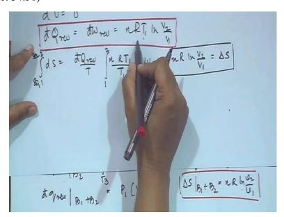
Compared this with the del delta s that you had obtained for an isothermal process, what do you find? You find that the delta s for both the cases are the same but we find that the dq for this process and the dq for this process they are not the same.
