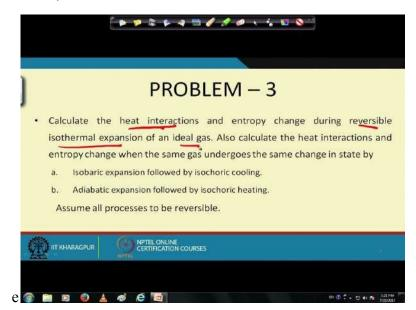
But this was pretty simple but the problem does not end here we are required to find out the heat interactions then the entropy changes for 2 other processes which provided the initial and final states are the same. What are the 2 other processes? The 2 other processes are isobaric expansion followed by isochoric cooling, adiabatic expansion followed by isochoric heating and all the processes have to be reversible.
