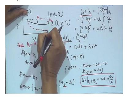
Again you can repeat it for the next process which is given, the next process is nothing but your adiabatic expansion, say for the next process what is it? This is basically the adiabatic expansion followed by the isochoric heating. So therefore here we start from P1V1T1 along a process say
