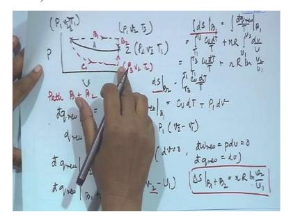
And we can also for this particular path C1, say for this particular path C1 we can also write that CvdT equals to minus nRt dv by v, why? Because du equals to minus w since dq equals to 0, right? So therefore instead of the CvdT by T, can we not substitute it with minus V1 BY V2 nR dv by v, which gives us minus nR ln v2 by, in this particular case there was a minus, very sorry so it becomes a plus so therefore this is ds in this particular case, right?
