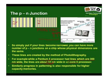
Photolithography is something that we will probably take up after 2 or 3 lectures may be a little later, this is what is known as Photolithography, but it is extremely important from the stand point of micro electronics industry and this is sort of a silicon electronics as it is called photolithography is the industry standard or the only technique for creating these semiconductors or these basic this p-n junctions, which are absolutely essential for making the computer chips or the processors.
