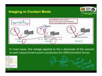
So, this particular slide should know make sayings you all of you, it is essentially some sought of a very enterprise schematic of a constant force contact mode imaging and this moves from point 1 to point 2 essentially in to the during the rastering. And we also now understand it is the piezo electrics scanner that essential takes care of this movement.
