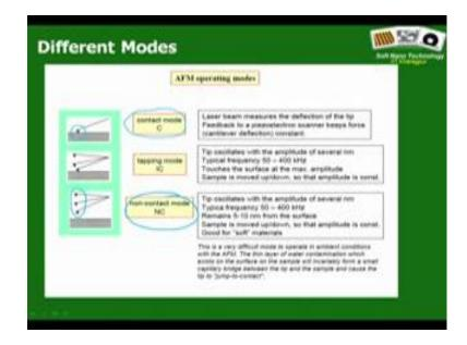
So, contact mode you already know where you there is no oscillation, you simply bring in the cantilever in contact with the sample surface. Typically in non contact mode classical non contact mode, what you do? You bring the cantilever very close to the surface and then start oscillate you need at in resonance frequency, you can choose the amplitude, but you choose the amplitude in such a way that the cantilever does not touch this surface right.
