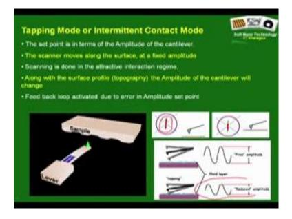
So, this now should be clear to you, this the zone corresponding to the free amplitude this gets truncated, actually get truncated from one of the site. So, it is reducing amplitude and you have a set point and based on that some point to point the amplitude is maintains to be constant.
