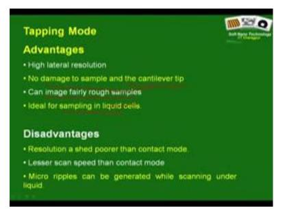
So, advantage pretty high lateral resolution no damage to sample and to the cantilever tip can image fairly rough samples and ideal for sampling this is wrong; in fact ideal for sample sampling soft images.
