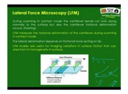
So, now what happens? What happens is though you have been talking or even in this image shows that a tip sought of is moving in this direction just like that, reality is you are. In fact, the dragging your tip during this restoring action over the surface and please do not forget that the tip is in contact with the surface and it is the scanner because of the contraction or expansion of the piezo that wants to move.
