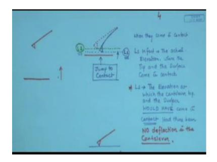
So, this was the cantilever, surface was far away, let us say the surface is moving up and now the surface is close enough to the cantilever. So, ideally this was the initial configuration of the cantilever, but what happens is because of this attraction in the surface attraction, the cantilever now feels the attraction and bends like this because your cantilever material is such that it deforms to the magnitude of Van Der Waals forces.
