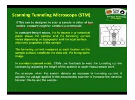
So, how does an STM work? Well STM in fact, works let us read what is written there. I am going bit slowly because it is a completely new topic. So, STM can work in two modes, let us read and then we will understand it is very simple either it is a constant height mode or constant current mode.
