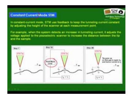
So, a better option is the constant current mode. Where there is an additional hardware element and that is a feedback controller. I think I am running out of time in this particular class. So, in the next class I will start from here and then move on to an AFM.
