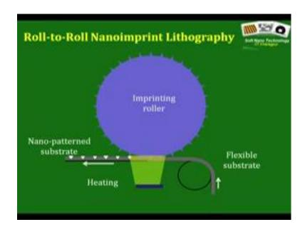
And there are very critical issues, but roller Nano imprint lithography works very well with flexible surfaces, but there are very many critical issues like the temperature as to be very accurately controlled and the viscosity should be absolutely appropriate the contact time should be absolutely accurate here.
