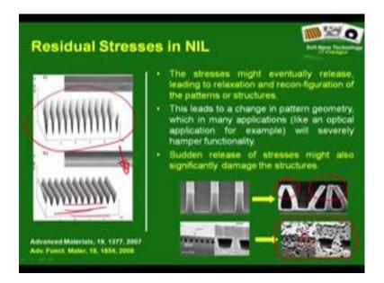
And will anything with stress is not good humans. Doctors always tell you reduce your stress same thing is valid for Nanostructures. So, if you now use it for prolonged usage. One notices that the structures tend to flatten out. One can see this type of tracks or sort of bearing like this which is all signatures of this release of this stresses of course, this flattening is not fully attributed to stresses it is also attributed to the reduction of the surface area or slumping phenomena.
