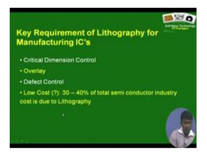
Key requirement of lithography for manufacture integrated circuits; so critical dimension control, overlay defect control cost because please do not forget the process are ruffle 30 to 40 percent of process are cost actually is due to lithographic process.
