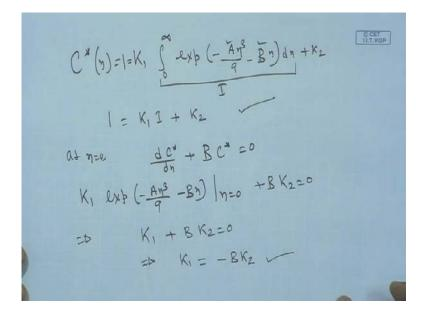
Now, with the help of these two one can evaluate the constants K 1 and K 2. So, if you do that, so, this become C star eta is equal to 1, so, this becomes K 1 0 to infinity exponential minus A eta cube by 9 minus B eta d eta plus K 2; so this is a definite integral because A is constant B is constant, so, we call this constant as I, so, 1 is equal to K 1 I plus K 2.
