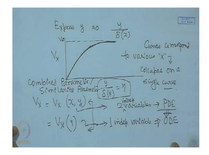
This curve and all these curves will super impose on one another and we will be getting a single curve. In this case we will be getting a single curve. so by doing a Therefore, all these curves will collapse. Curves correspond to various x; collapse on a single curve.
