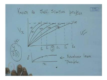
If we express y as y by delta which is nothing but a function of x and if we plot V x as a function - as this quantity y by delta, that means we are normalizing this axis by the corresponding deltas. This is delta, delta delta; but each delta is a function of x.
