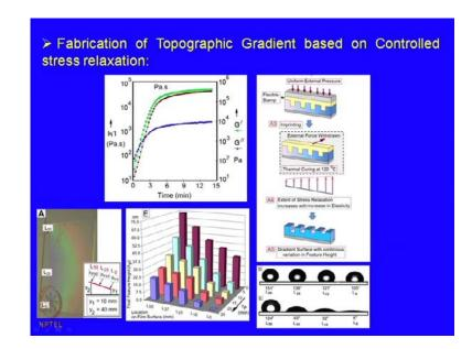
So, it is because of this this typical rheological response you can see for a sylgard. So, with time it is a progressive cross linking. So, which translates in our case to the fact that the thought of the film which have receive more heat sort of is higher cross links states for a elasticity is higher therefore, the stress relaxation will be higher there.
