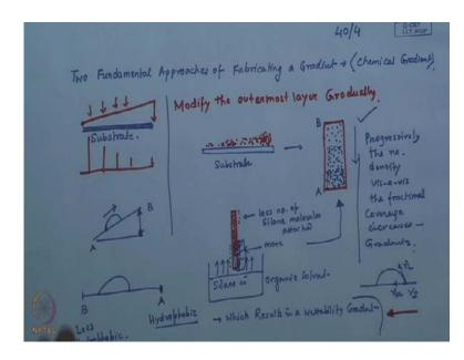
I am sorry cannot pronounce the the name of the silent properly in paraffin oil and let it evaporate. So, all the did was this was the bath which contain the the silent in a organic solvent. And the surface which was to be silenced was simply kept like this. So, as the
