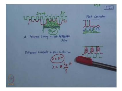
Now becomes r m is function, lambda is an a function of R F into H, and this R F tailored between any values between 0.5 and 8 depending on the configuration of the elastic bi layer, and which becomes a function of the ration of the share module I of the
