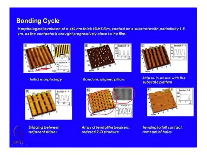
And if you now do an approach sequence, you see that the morphological evolution sequence is almost the same, you again see the array of holes appearing in this case and this optical micro graph shows how well organized and large area these structures are. So this is the morphology of the initial film.
