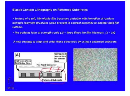
So, same thing happens here, if you now use a patterns substrate an on to which you coat your elastic film you have undulating a film with an undulating top surface and therefore, the inter surface separation distance over here, over these locations about the undulation is lower as compared to other areas, so this is expected to give a sort of a some sort of directionality preferential directionality.
