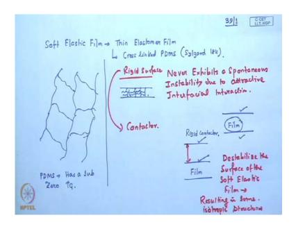
So, Soft Elastic Film essentially we are talking about a thin Elastomer Film, and we have actually talked about an Elastomer in pretty good detail while talking soft lithography. It is essentially a cross link PDMS is a perfect example of a Elastomer thin film.
