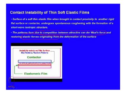
So, the pattern essentially form due to a competition between the attractive Van Der Waals force acting between the free surface of the film, and the Contactor so again the Van Der Waals force again the attractive Van Der Waals force is present but the forces is not active between the two interfaces of the film but it is between the Contactor and the film, and any instability is essentially opposed by surface tension as well as elastic forces originating from deformation of the matrix.
