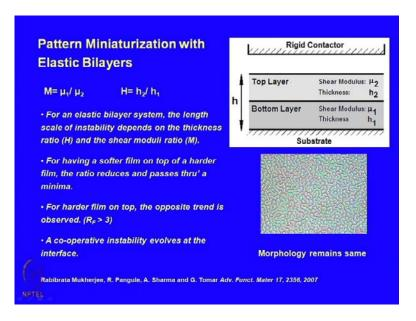
And when the film thickness is much higher it completely sort of disobeys the presence of the substrate pattern, and you get these labyrinth. The other interesting aspect is that, you can tailor this lambda equal to three h scaling by using an elastic bi layers where this scaling ratio.
