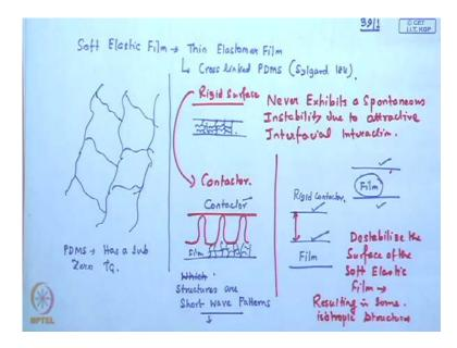
So, what happens is now you are looking at a system, so suppose the film involves like this, we will immediately see so this a Contactor let say which is coming in contact, the film become unstable makes an structures with sort of tend to go and touch the Contactor.
