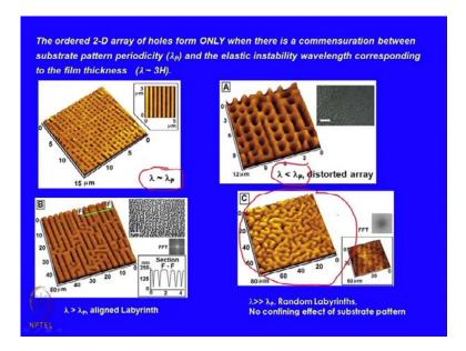
So if there is commensuration, you get an aligned perfectly aligned array of this 2 D holes, slightly lambda slightly lower than lambda p de sorted array lambda higher than lambda p you tend to back to the align structures but labyrinth but they sort of align because of the presence of the subsurface substrate pattern substrate or align substrate.
