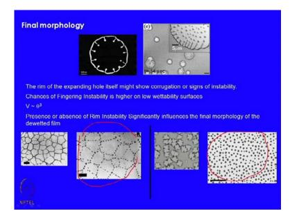
So this is, if you have a rim instability or fingering instability this is the lightly morphology to get. You get a completely random array of the droplets, in contrast in cases where there is no rim instability; it is lightly that your droplets will be arranged like this.
