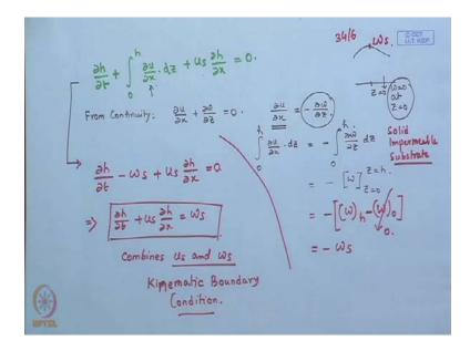
Then, what you get in the final form is that, del h del t plus integral 0 to h del u del x into del z plus u s del h del x is equal to 0.
