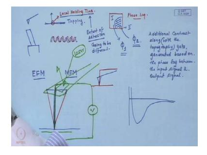
So, next week (()) to the other class of techniques, these are particularly EFM and MFM I should focus, I should mention, that is, the electrical force microscope and magnetic force microscope. These are very unique techniques, which sort of, allow you to identify either distinct electrical domains based on long range Coulomb forces, by taking advantage of the Coulomb forces or magnetic domain, by taking advantage of magnetic interaction.
