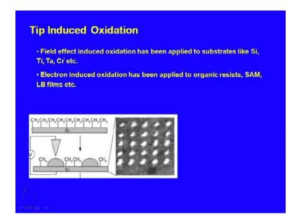
One can also use this concept for, let us say, something like a tip induced filed effect, tip induced oxidation on surfaces like silicon, titanium, (()), chromium, etcetera. So, electron induced oxidation has also been applied to organic resists and something like that. So, it is a combination of electrical force measurement and righting.
