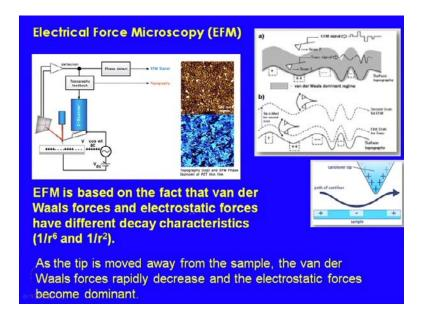
This nature of the curve might change, but what you need to understand, that this columbic forces for example, so this columbic force, electrostatic forces have a much reduced decay characteristics as compared to Van der Waal's forces. So, let us say, between particles Van der walls forces 1 by R to the power 6 and we know that and coulomb forces 1 by R square.
