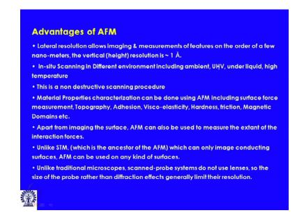
So, that sort of brings to the last line and last couple of slides soft of this class of this topic, the advantages of AFM. So, one can achieve lateral resolution allowing imaging and measurement of features and order of few nano meters, and the vertical resolution can he as low as one Angstrom, one nano meter vertical height, of course, it is almost possible to achieve in any standard AFM.
