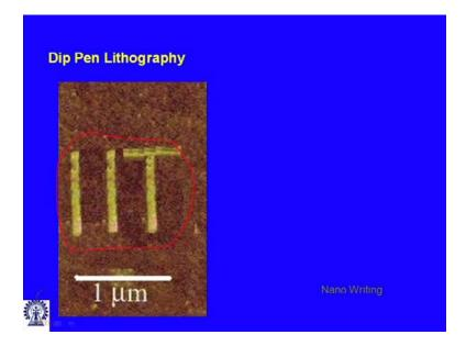
So, this is what in a nutshell is dip pen nano lithography. So, here you can see, we wrote something using silent molecules, of course this is a little wider, roughly about 80 nano meter width. So, there are multiple movements, so that to make it visible.
