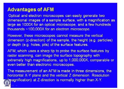
So, same things, it is sort of a comparison of AFM with other class of microscope or optical or electron microscopes. So, optical and electron microscopes can easily generate two-dimensional images of a sample surface with magnification as large as one million times for an electron microscope.
