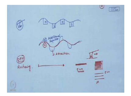
So, exactly in the same way one can, one needs to know what type of tip one is using, whether it is N or S and we might be having surface topography with this type of different domains. So, you do a contact mode scan and then, you do a non contact scan to find, that there are certain zones where it is deviating.
