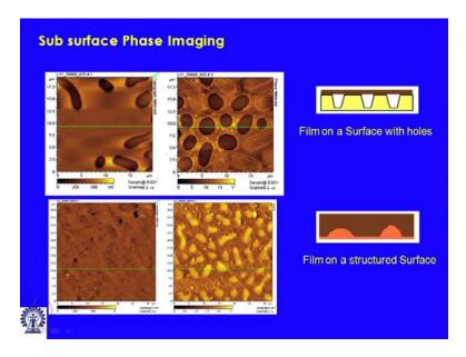
This is couple of example. So, this is how sub surface structures can be sort of imaged using, based on the phase imaging. So, this is a special example we had a sort of a holy surface and surface at some holes and which we have coved with a thin polymer film like this.
