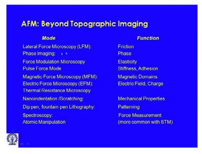
There are a whole lot of things, that can be done and also, before I forget I must mention, that in adhesion to imaging, the rastering action can also be, to some extent, used in patterning technique as one of the direct write patterning technique and in most cases, this is what is known as or referred to as the DPN or the dip-pen nano lithography operation. So, we will talk about some of this and some of the secondary imaging modes of an atomic force microscope.
