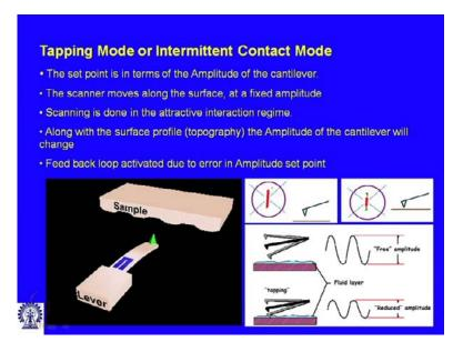
So, this is how, sort of tapping mode works. So tip vibrates close to the sample surface, five to fifteen nanometers away with an amplitude hundred to ten nanometer, and this cartoon will give a nice idea about the taping mode. So, here you see the, this is the moment of the laser path, as a corresponding to the free amplitude oscillation, and this is far away from the surface, and since the surface is now close it is sort of gets truncated. I
