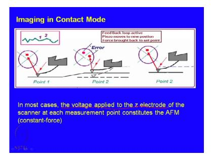
So, in most cases, the voltage applied to the z electrode, z direction of the scanner, at each measurement point constitutes the A F M data, we will discuss this in later detail.
