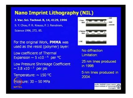
So, this is what we showed in the previous class the method is very, very simple, all unit do is to sort of take a hard rigid stamp which as the structure, a negative replica of the structure
