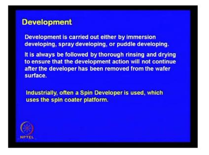
So, development is carried out either by immersion developing, spray developing or puddle developing. It is always be followed by thorough rinsing and drying to ensure that the development action will not continue after the developer has been removed from the wafer surface. Industrially, often a spin developer can also be used which typically uses the spin coater platform.
