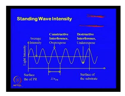
So, this is exactly what is suppose this is the surface of photo resist. So, this is now you have the photo resist film, between let us say these two inter faces, this is the photo resist here interface and surface the photo resist oxide inter face. So, you this particular graph.
