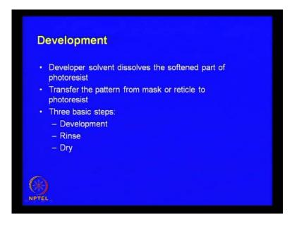
So, a development solvent dissolves the softened part of photo resist, transfer the pattern from mask or reticle to the photo resist. And three basic steps are development, rinsing and dry. We will pick up the later part of the concluding part of photo lithography in the subsequent class.
