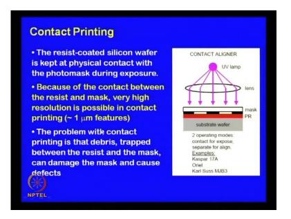
So, let us looking to it in little big detail, this is very, very simple. So, you just take your mask, you just place it in direct contact with the photo resist layer, if there is no dust particle or any other defect these two will coming (()) much conformal contact, because the mask and the film both are smooth.
