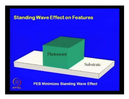
So, this is the average intensity of light and what happens is due to constructive interference and destructive interference, some areas across the depth will get overexposed, some areas will get underexposed. This results in this type of a standing wave effect on the features. Your post exposure bake actually take care of this standing wave effect and because of that is annealing, it minimizes the standing wave type of structure.
