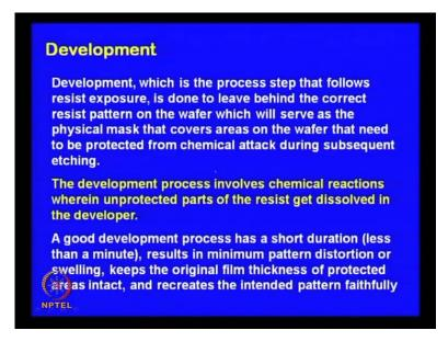
So, once post exposure is done then the next stage that the final stage I would say is the development which is the process step that follows resist exposure is done leave behind the correct resist pattern.
