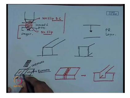
So, this is the stage where using a mask like this. So, this is the unexposed areas and this is the exposed areas. So, it is this stage the developer solution so as we told initially, but every photo resist sort of comes with it is own developer solution. So, suppose if it is a positive photo resist then your developer solution will wash away these zones. In contrast, if it is a negative photo resist the developer solution will only wash away these zones.
