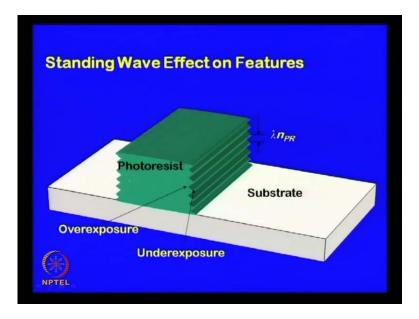
So, what happens again is due to interference of the different wavelengths, what eventually it result is the standing wave effect on the feature. So, because of this interference, the intensity sort of varies like this which get replicated on the photo resist layer. So, you have you get the structure like this.
