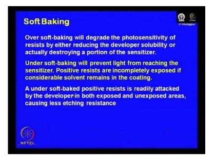
Now, couple of things that over soft baking will degrade the photo sensitivity of the resist, by either reducing the developer solubility or actually destroying a portion of the sensitizer. We already know that a photo resist has sensitizer, which is essentially responsible for the photo active properties and if you over bake it due to the prolonged
