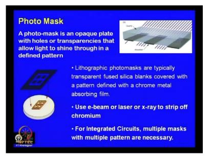
So, now it brings us back to a slightly detailed discussion or if the stage is now, right for a slightly detailed discussion of what a mask is or a photo mask as it is ideally called is, so essentially a photo mask is an opaque plate with holes or transparencies that allow light to shine through in a defined pattern.
