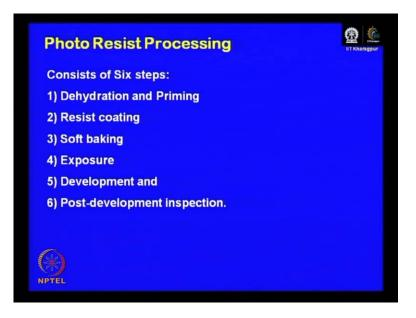
So, now let us get back to the photo resist processing steps. You now understand that the base material, this processing is going to be with photo resist.
