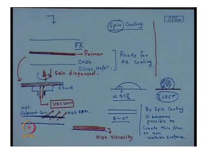
So, now you have an oxide coated, and primed limit, moisture removed, and primed wafer which is now ready for photo resist application. So, this is now ready for PR photo resist coating or photo resist application.
