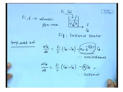
Now, the schematic representation of an isothermal C S T R is like this inlet flow rate is F i concentration is C A i, the output is coming out with a flow rate of F and A concentration of C A. So, the concentration in the vessel is also C A and will assume the value is V, since there is no variation of temperature. So, there is no need of any external heating or cooling medium.
