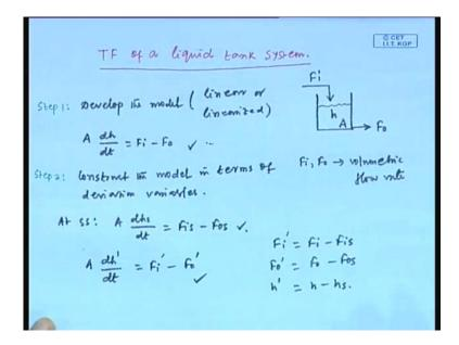
So, we will derive the transfer function of a liquid tank system. So, this is a schematic of a liquid tank system, a liquid is entering at a flow rate of F i and the output is coming out at a flow rate of F naught. The liquid height is h cross sectional area of tank is suppose A. This is a schematic of a liquid tank system, F i and F naught both are in terms of volumetric flow rate.
