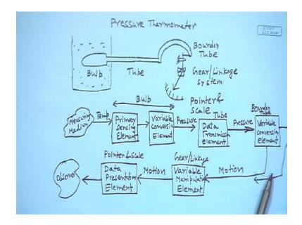
Let us redraw the figure here; you have the bulb of the bourdon tube, bulb of the pressure thermometer. Then the tube and a bourdon tube disconnected for simplicity, let us draw a c type bourdon tube. So, this is bulb, this is the tube or capillary tube, this is the bourdon tube, this is gear and linkage system, this is pointer and scale and this is bulb is put to the medium which temperature I want to measure. So, you can put to a see breathable liquid is temperature we want to measure.
