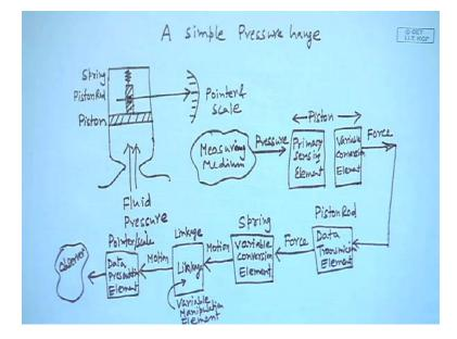
Will take a very simple pressure gage, which measures will pressure of a fluid and the measure pressure is indicated by deflection of the pointer against the scale. Consider a
