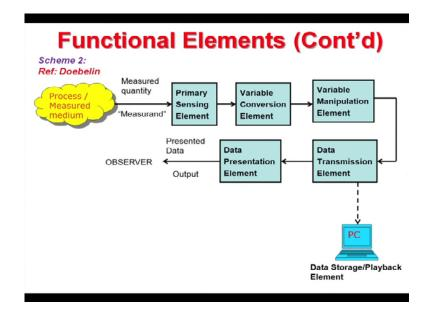
Let us discuss another scheme as proposed by doebelin we have a process or measure medium as before again consider it is liquid whose temperature I am going to measure. So, I bring a temperature measurement measuring instrument in contact with this measure medium and analyze how the instrument works I mean able to identify these functional elements.
