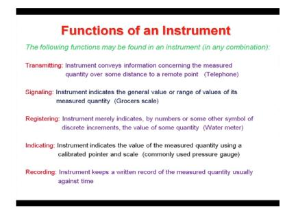
Well the instrument measures the value of a condition the following functions may be performed by an instrument transmitting signaling registering indicating and recording accordingly, you can say transmitting instrument signaling type of instrument registering instrument indicating type instrument and recording instrument.
