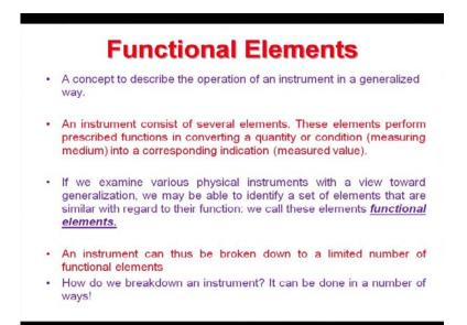
Now, let us come to an important concept called functional elements is a very useful concept to describe the operation of an instrument in a generalized way an instrument consist of several elements these elements perform a prescribed functions in converting a quantity or condition which is measuring medium into a corresponding indication which we called measured value.
