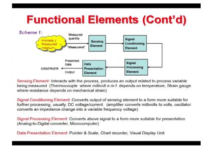
Let us look at this scheme which describes how you break down an instrument into various functional elements you have a process or measured medium which i am interested in measuring having a instrument in contact with this the instrument interact with this measure medium and presents may what it has measured.
