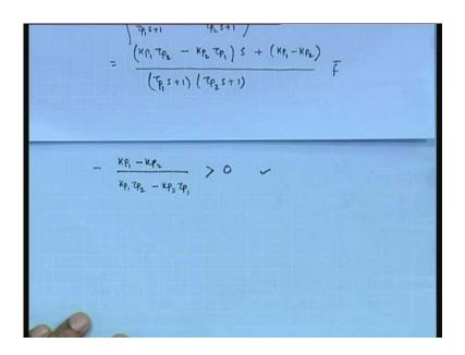
Minus K p 1 minus K p 2 divided by K p 1 tau p 2 minus K p 2 tau p 1 this is a 0 agree. So, what is the condition for inverse response behavior? This 0 should be positive; that means, the condition is this should be greater than 0, this is the condition for inverse response behavior. Next, we will implement the controller i mean we want to develop the closed loaf block diagram.
