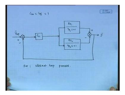
So, our process has the transform function of K p 1 divided by tau p 1 s plus 1 and K p 2 divided by tau p 2 s plus 1 with opposite effects. The transform function for the
