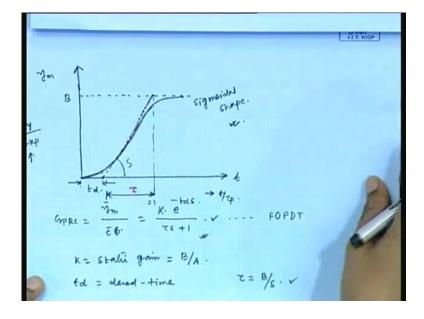
Now, can you find the expression for k change in output that is B divided by change in input that is A agree, gain is the change in output divided by the change in input. Next one is the t d, t d is date time, date time value you can obtain from this plot, this is the date time. Date time value we can obtain from the plot. Now, if we exclude the date time plot, then the response becomes the response of the first order system. If we exclude the
