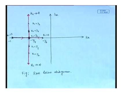
With the increase of K c value, the poles of the closed loop system they move away from the real axis. See here, this root we got when K c equals one fourth, if we increased to K c half, the root is moving away from the real axis in both sides what it indicates, oscillatory response
