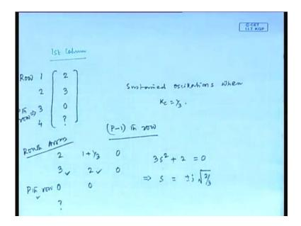
First element is 2, second element is 3, third element is 0 so, upto third row, we can determine the elements in the first column. If the elements in the third row vanish then what about the close loop response, we have discussed in last class, sustain oscillation. So, if all the elements from the third row vanish then we can conclude that, the close loop response provides sustain oscillation I mean, oscillatory response with constant amplitude.
