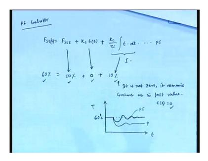
PI controller as long as the error is present the PI controller keeps changing its output by integrating the error. If, we see the controller equation Fst equals Fst s, plus proportional term Kc epsilon t plus integral term; that means, Kc divided by tow y integration error dt. This the PI controller equation. So, this is the integral term as long as the error is present the PI controller keeps changing its output by integrating the error.
