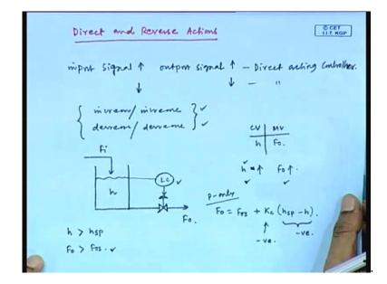
We will discuss next Direct and Reverse Action. So, as the input signal to the controller increases the output signal from the controller should increase for direct acting controller you note down this point, as the input signal to the controller increases the output signal from controller must increase.
