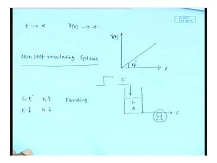
Now, we will represent it graphically, if we consider t tends to infinity what happens y t tends to infinity. So, this is y t and this is time t this is the output and slope is k p prime. This type of processes are called non self regulating processes, this type of processes are called non self regulating systems. Question is why, we will consider one system, that is liquid tank system, to explain this concept we will consider one liquid tank system.
