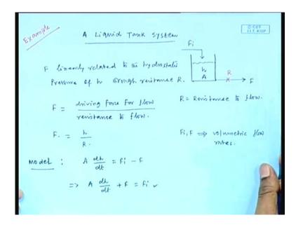
We will first consider one example that is a liquid tank system. Will consider a example that is a liquid tank system. This is a liquid tank height of this liquid is h, cross sectional area of the tank is suppose A, input is entering the tank with a flow rate of f i and output is f and here, we are considering resistance that is R. Now, this effluent flow rate f is related to the hydrostatic pressure, of the liquid height h through resistance R, here R is the resistance to flow.
