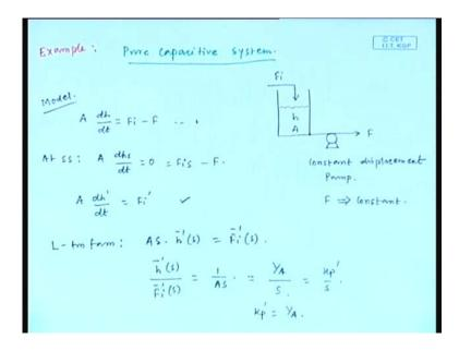
We have consider another example, that is the example of pure capacitive system I mean how we can get the A naught y term equal to 0 physically, we will continue the liquid tank system, which we considered earlier. So, this is a liquid tank system height is h, area is A inlet flow rate is f i in the outlet section one pump is installed, which is delivering outlet with a flow rate of f.
