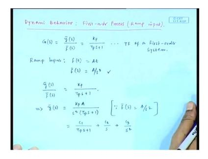
So, next topic is dynamic behavior and we will consider first order process and we will change the input as ramp function, I mean the input is ramp input. This we will discuss in the next. So, we have already derived the transfer function of a first order system in general form, that is G s equal to y bar s divided by input that is k p divided by tau p s plus 1 this is the transfer function of a first order system.
