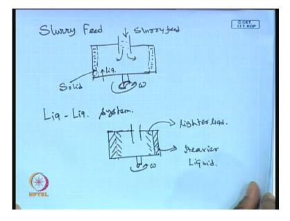
So, for slurry feed, you will be having, and the central the bowl will be rotating about the central axis with a speed omega, and the slurry will be coming and the solid particles will be experiencing a force. So, centrifugal force towards the wall so therefore, they will be depositing over the walls. So, you will be getting a layer of solid particles there, and this will be the liquid and you will be having solid particles there.
