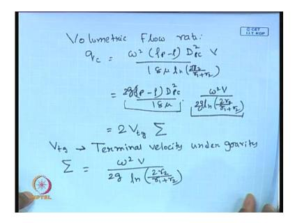
Let us let us look into the volumetric flow rate, volumetric flow rate is given as q c is equal to omega square (rho p minus rho) D p c square V divided by 18 mu l n (2 r 2 divided by r 1 plus r 2). Now you so, just separate these two out, so I will be I will be taking the geometric and the operating conditions on the right hand side, (rho p minus rho) D p c square divided 18 mu multiplied by omega square times V l n (2 r 2 divided by r 1 plus r 2).
