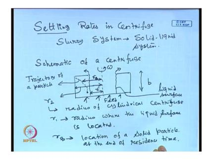
Now, let us look into the settling rates in centrifuge, now we are talking about let us say, talking about a slurry system, and always slurry system it is basically, solid liquid system. In that, so let us first draw a typical centrifuge, so you draw a schematic of a centrifuge, then all our nomenclature will be fixed; so we are having the liquid surface, and the whole system is rotating about its central axis with omega.
