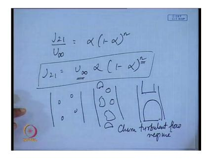
Normally what do we say? We say that for the bubbly flow pattern we have bubbles of this sort. For the slug flow pattern we have something of this sort. Now, for the churn turbulent flow pattern we can have a wide type of bubbles, we can have cap bubbles it can be a totally erratic distribution resembling the churn flow regime to some extent. So, therefore, usually this particular flow pattern which is the transition between these two this is usually known as the churn turbulent flow regime.
