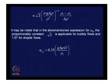
And this particular equation is for the slug flow pattern. So, for different flow patterns we have different particular flow equations or rather different expressions of drift velocity.
