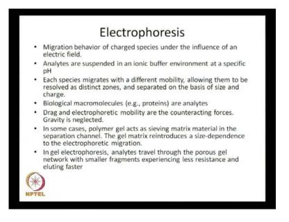
This basically separates a mixture of particles based on their size and charge they ban them in in layers and then these layers can be eluted in the way you want.
