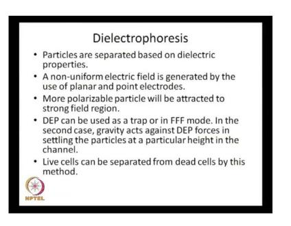
The next item that I want to discuss today is known as Dielectrophoresis. This is little different from electrophoresis. Here, particles are separated based on dielectric properties not their size and charge. Particles are separated in electrophoresis particles are separated based on their size and charge. Here, in dielectrophoresis the the whole idea is
