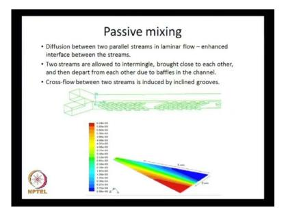
Then this we wewe discussed about mixing you remember that mixing would be an essential part because you are introducing a sample and very importantly that sample has to mix with the reagents that sample has to mix with the reagents. So and then how it responds to certain reagent that you are checking in the detector.
