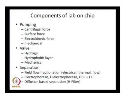
We mentioned in the last class that you need to have a pumping action, a valve action, a separation process going on, mixing, heating, detection all these happening inside the chip.
