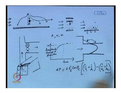
So if this is two third, then this is 1 third.So what you are doing essentially is if this is the this is the one you have and half of the stream was a and half of it is b and they are fed into the channel then this groove is basically starting one one groove is starting from here and that is the groove and the other groove is in this direction so you are basically swirling you you have taken 2 third and you are swirling here and 1 third you are taking
