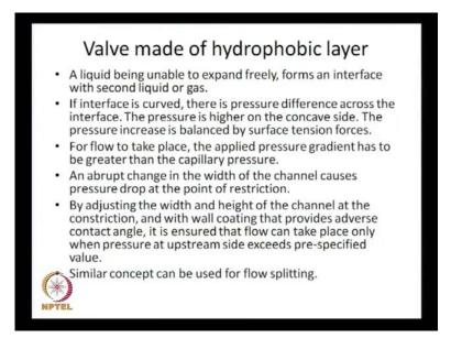
Then, this other idea that is there wall made of hydrophobic layer. It is basically something like this, a liquid being unable to expand freely forms an interface with second liquid or gas that that is basically the essence of surface tension. If interface is curved there is pressure difference across the interface the pressure is higher on the concave side and the pressure increase is balanced by surface tension forces. How would I put it here?
