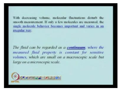
And we would see that how this is going to affect the the the continuum hypothesis. So, when we start reducing the volume, the molecular fluctuations would start to disturb the smooth measurement. So, you are not going to get a one value of pressure, but you would rather get a fluctuating pressure that can vary widely from one instant to another.
