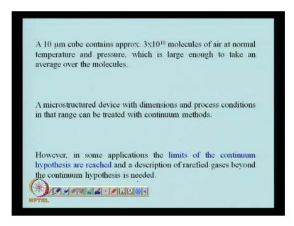
So, let us say we take a take air and we try to see, the number of molecules which are present in air at normal condition. So, you think about a 10 micron cube, instead of the one micron cube example that I have given you it is it is a cube found of 10 micron by 10 micron by by 10 micron. And if you calculate the number of air molecules present in such a cube at normal pressure and temperature, you would see the air of the order of 10 to the power 10, so it is a huge number of molecules.
