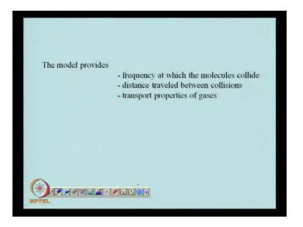
So, this model essentially provides us with a frequency at which the molecules are going to collide, the distance which are traveled between collision and the transport properties of the gases and there is to something else to see is that, this also tells us like, what will be the effect of the temperature.
