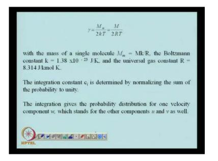
And this integration in this integration constant can be evaluated and one can obtain the integration constant by normalizing the sum of the probability to unity. And therefore, you can obtain gamma from the kinetic theory the and this is the relation for gamma and the integration constant can be obtained. So, this integration gives the probability distribution of one velocity component which is w, the other components in other direction u and v can be calculated in a similar fashion.
