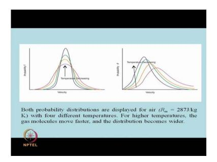
So, these two are well known figures where the probability is plotted against velocity at different values of temperature and you can see that the probability distributions, these probability distributions are for air and for higher temperature, the gases are going to move faster and the distribution is going to be wider and wider. So, these are at higher
