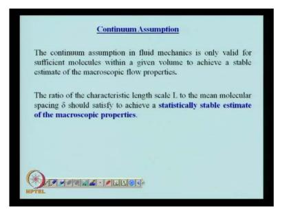
So, the continuum assumption in fluid mechanics is only valid when you have sufficient number of molecules present in a given volume so that you achieve a stable estimate, stable which is which is not, where there is not fluctuations of the microscopic of the macroscopic flow properties.
