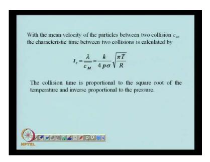
And finally, when we know the mean free path of the particle mean velocity particles between two collisions, the characteristic time between two collisions can be evaluated and as you can see, the collision time is proportional to the square root of temperature and inversely proportional to the pressure.
