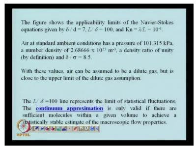
And if you think of air, you would see that it has a number density at 1 atmosphere pressure of 2.6 into 10 to the power of 25 in a meter cube size and density ratio which is about 8.5. So, with these values, one can say that air is a dilute gas, but it is close to the
