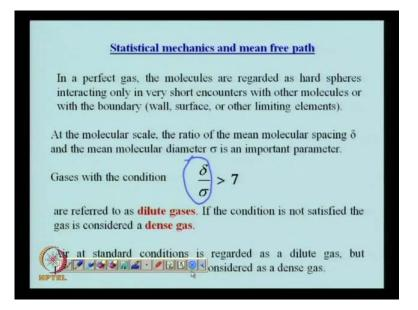
Now, we come to our next part which is the statistical mechanics and mean free path, usually gases with this condition that delta by sigma greater than 7 where delta is the mean molecular spacing. And mean molecular spacing and sigma is the main molecular diameter, this is going to be an important number, delta by sigma and gases with the condition delta by sigma greater than 7 are treated as dilute gases and if the condition is not satisfied, then the gas is called dense gas.
