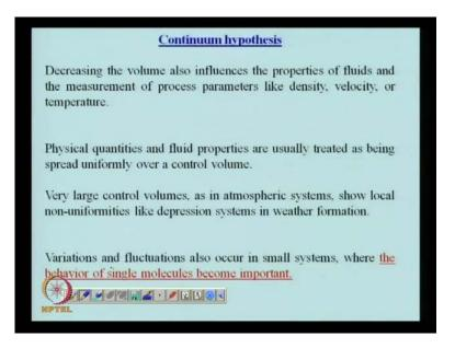
Now, what is continuum hypothesis? If we if we if we start reducing the volume, it is of of any system at some point of time, it start to influence the properties of the fluids and the measurement of process parameters like density, velocity or temperature will be affected by the reduction in size of the reduction size of the system.
