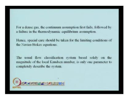
And so, one should take a special care for the limiting conditions to use, the limiting conditions of the Navier-Stokes equation and as the you can see now that the Knudsen number, the magnitude of the Knudsen number is just one parameter, one of the many parameters, one of the 4, 5 parameters which I have mentioned that describes the nature of the system.
