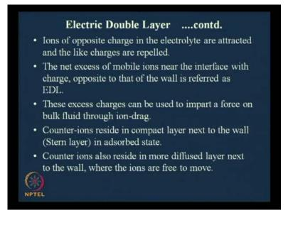
Now, this once there is a surface charge acquiring, one once these charges are acquiring on the surface or acquired on the surface, then there would be opposite charges getting attracted. And this is forming an excess of mobile ions near the interface with charge, opposite to that of the wall, and this is referred as electric double layer; these excess charges can be used to impart a force on bulk fluid through ion-drag.
