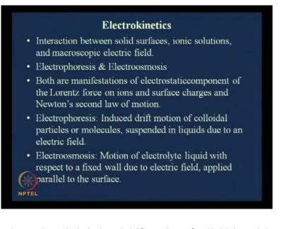
You remember, electrophoresis is induced drift motion of colloidal particles or molecules suspended in liquids due to an electric field. So, what we have is, we have an electrode here, we have another electrode here, and we have a particle we have a particle here (Refer Slide Time: 51:21). Now, this particle has certain charge in this and you have already imposed an electric field, you have imposed an electric field E and this particle has charge q.
